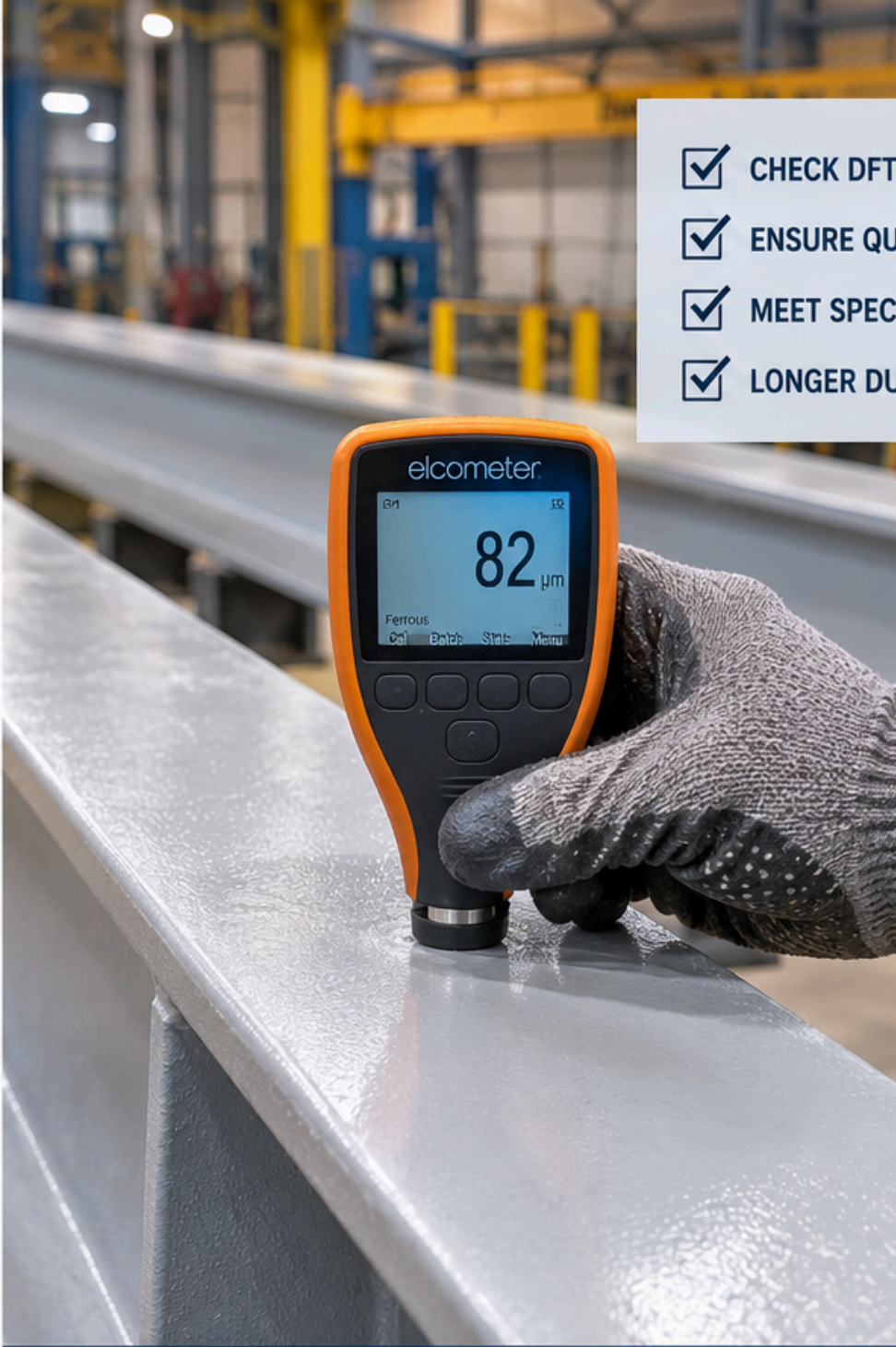
DRY FILM THICKNESS (DFT) MEASUREMENT RIGHT THICKNESS | BETTER PROTECTION | LONG
